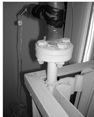
(b) Frost type near outlet of the vaporizer (crystal frost type)
