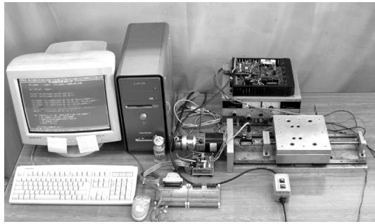
Fig. 4. Photograph of the servo position tracking control system.
