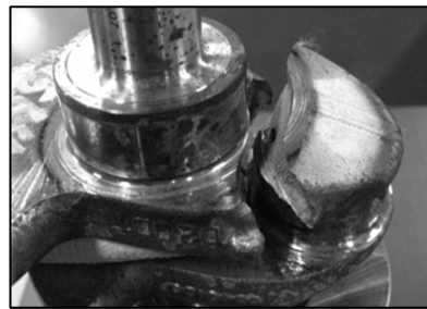
Fig. 4. Failure mode during bending test.
